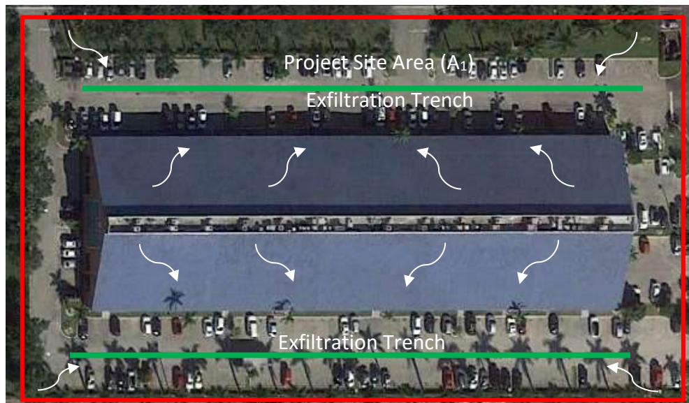
Figure 7.1 - Area Attributed to an Exfiltration Trench Length
