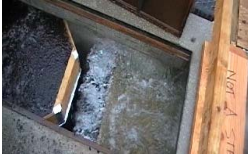
Figure 2. View of Inlet/Outlet Bay and a portion of the StormFilter Bay at 57 l/sec (2.0 cfs), 56 seconds into “instant-on” test. This image shows hydraulics once system has filled.
