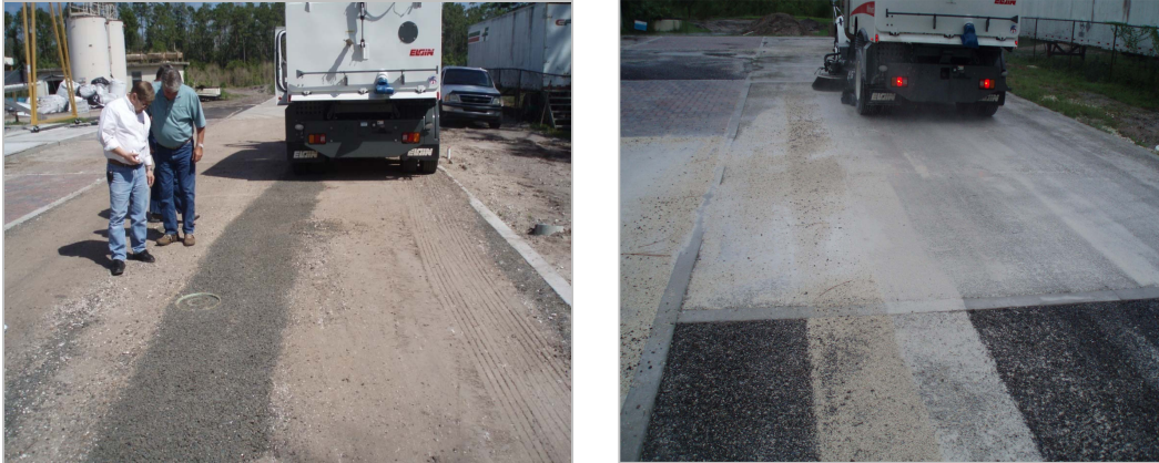
Figure 3 (a) Vacuum sweeping of sandy sediment loaded surfaces (b) vacuum sweeping of fine limestone dust loaded surfaces
